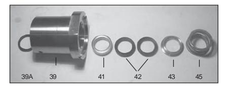
11. Take a thin screw driver and pry out the grooved ring (39A). Note: This seal (39A) will not be reusable, so replace with a new part. For the seal-pack (41-43A), remove with either a socket wrench or use a screw driver to push against the rear lip of the pressure ring (41) or v-sleeves (42). You will need to remove seals evenly out of the seal sleeve (39). Be careful not to score the sleeve or metal parts (41 & 43).
